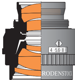
Optical design (105 mm f/4): 7 elements in 6 groups
