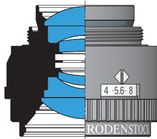
Optical design (80 mm f/4): 6 elements in 4 groups
